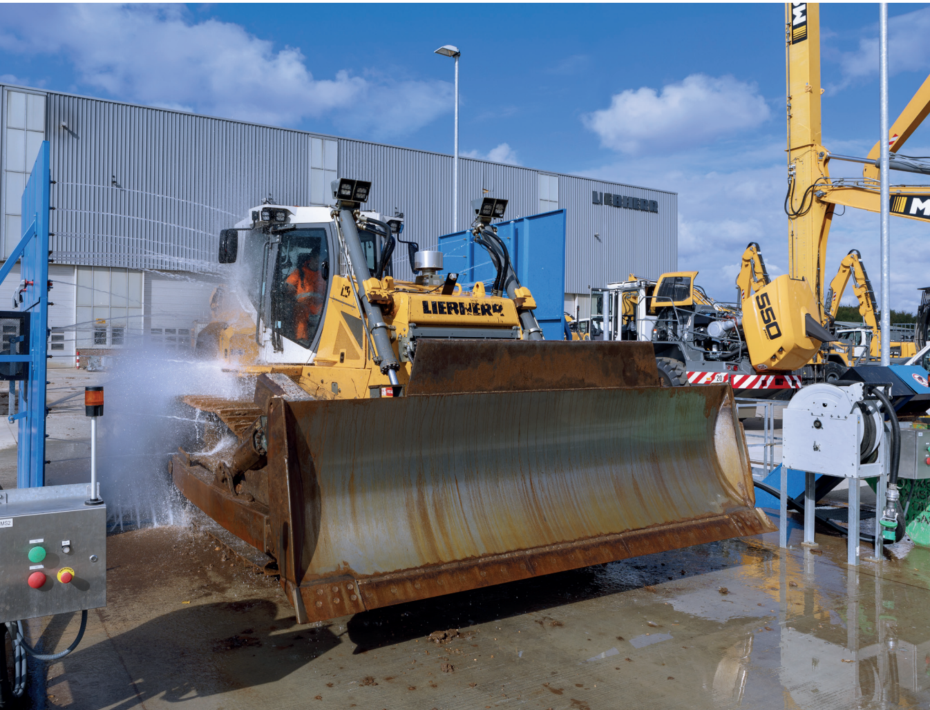
HD - Automatische Grobreinigung in wenigen Minuten HD - Automatic intensive primary cleaning in a few minutes
